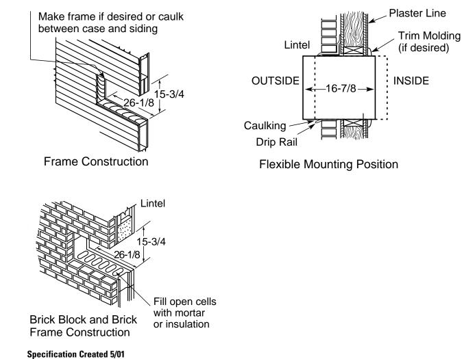
Installation Information: A finished opening of 26-1/8" x 15-3/4" clear of intrusions is required. Keep clearance of 4" from side walls. Brick veneer or frame walls should have wood studding surrounding case to provide firm anchoring with screws. Case can be fastened directly to brick or block walls with screws sunk in lead expansion shields.
