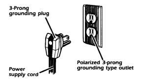
The compactor is for use on a 120-volt, 60 Hz, AC only 15 ampere fused and properly grounded circuit and is equipped with a grounding plug as shown above. For your personal safety, the compactor must be grounded. In the event of an electrical short circuit, grounding reduces the risk of electric shock by providing an escape wire for the electric current. This appliance is equipped with a polarized 3-prong grounding plug.
