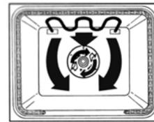
During convection broiling, the broil elements will cycle on and off in intervals to maintain oven temperature, while the fan constantly circulates the hot air.
