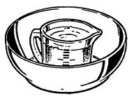
water—set the measuring cup either in or next to the dish. Microwave 1 minute at high. **If** the dish heats, it should not be used for microwaving. If the dish remains cool and **only** the water in the cup heats, then the dish is microwave-safe.
