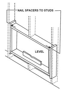
**NOTE:** If wall thickness is 8-1/2" or more, add aluminum flashing over bottom of frame opening to assure no water can enter area between inner and outer wall.
