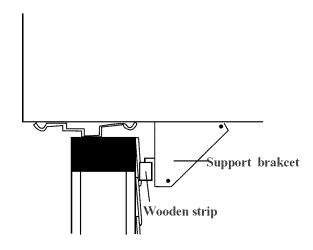
5. Screw or nail cabinet wooden frame using shims if frame is oversized, to eliminate distortion. Remember to maintain proper slope as described in Step 3.
