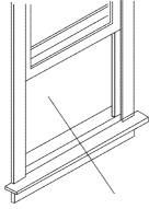
2. Place cabinet in window with bottom stool angle firmly scated over window stool as shown. Bring window down temporarily behind top angle to hold cabinet in place.
