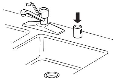
The drain air gap is usually located on top of the sink or countertop near the dishwasher. To order a drain air gap call your local dealer, or in the U.S.A., call the Customer Interaction Center at 1-800-422-1230 and ask for Part Number 300096.
