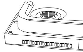
The vent closes during the cycle to lock sound in the dishwasher. After the cycle has finished, the vent remains closed until the dishes have cooled down. Between cycles, the vent stays open for air-flow, reducing the build-up of odors.
