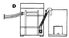
If a longer drain hose is needed, drain hose extension kit (Part No. 285702) is available from authorized parts distributors. If drain hose must be shortened, use hose kit (Part No. 285442).
