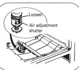
To adjust the flow of air to either burner, loosen the Phillips head screw and rotate the shutter toward open or closed position as needed.
