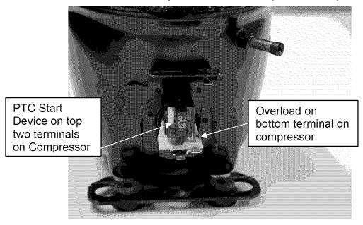
7. Install Wire Jumper included in kit on left terminal (number 1 on relay) of PTC Start Device as shown below.
