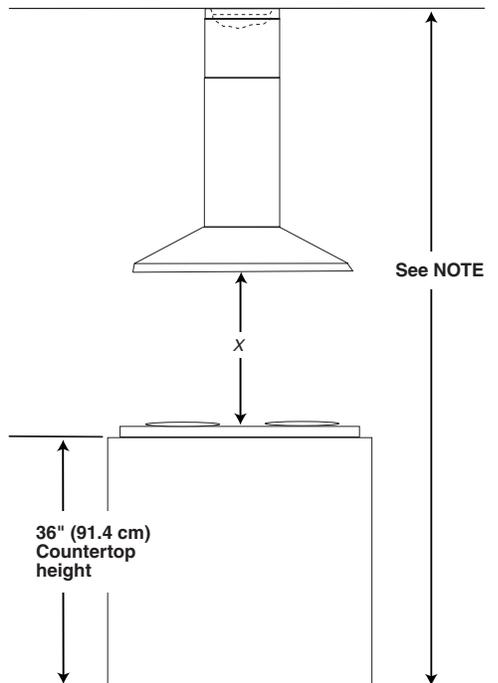
**NOTE:** The hood chimneys are adjustable and designed to meet varying ceiling or soffit heights depending on the distance “X” between the bottom of the hood and the cooking surface. For higher ceilings, a 40" (101.6 cm) Chimney Extension Kit Part Number 8212698 (Black), Kit Part Number 8212696 (Stainless Steel) or Kit Part Number 8212697 (White) is available. See your dealer. The chimney extension replaces the upper chimney shipped with the hood.
