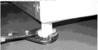
Press down on alternate corners and sides and feel for the slightest movement. Adjust the appropriate leg so the washer is SOLID on the floor on ALL four legs. Keep the leveling leg extension at a minimum for best performance of the washer.
