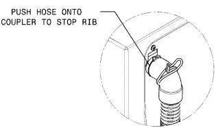
3. Using pliers, squeeze the ears of the spring clamp and position the clamp so the clamp ears <u>align with</u> <u>and contact the tabs</u> on the drain hose. This assures proper location of the clamp to prevent leaks.
