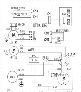
The wiring diagram is for explanation purpose only. The actual shape of the components may be different.
