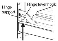
Lock engaged for door removal Figure 1
