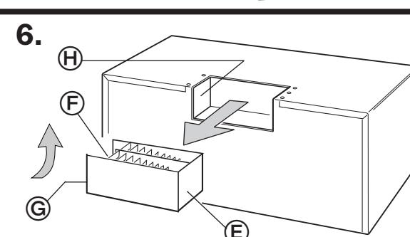
Slide air deflector back into cabinet as far as it will go. Check that deflector vanes **F** face the top of the cabinet and that the small exhaust ports **G** **H** face each other.
