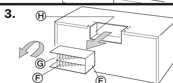
Slide air deflector back into cabinet as far as it will go. Check that deflector vanes **F** face the rear of the cabinet and that the small exhaust ports **G** **H** face each other.
