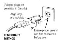
**A** CAUTION: Attaching the adapter ground terminal to the wall receptacle cover screw does not ground the appliance unless the cover screw is metal, and not insulated, and the wall receptacle is grounded through the house wiring.
