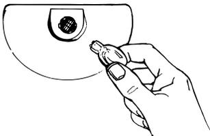
5. Replace the cutter grid cover with two screws.
