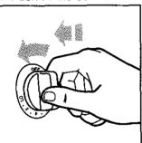
clockwise to the LITE position. The clicking sound is the ignitor sparking. Make sure the burner has lit.
