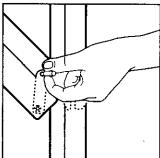
included with your range, into both hinge hangers. Do not remove the pins while the door is removed from the range.
