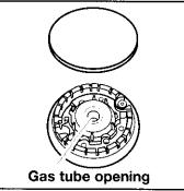
replace the burner cap. To replace the burner cap, make sure the alignment pins on the cap are properly aligned with the burner base.
