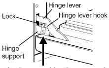
Lock engaged for door removal Figure 1
