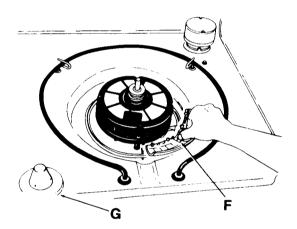
The coarse strainer may be removed, if necessary. To remove, lift strainer out by squeezing centre section (F) and remove. To replace, squeeze centre section so clips snap into square notch.
