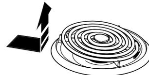
2. Pull the coil element straight away from the receptacle.
