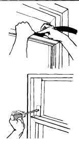
Insert window rail seal behind top of lower window sash and against glass of upper window. Place window-lock bracket on top of lower window and against upper window sash. Use a 3/32' drill bit to make pilot hole. Attach window bracket. Seal small openings around window with gumtype sealer.
