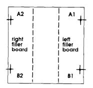
Subtract 1/8" from both open area measurements. Use a saber or hand saw to cut filler boards on the side opposite the holes.
