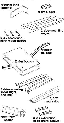
Installation parts are supplied for double-hung windows up to 38 Inches wide. Installation up to 54 Inches can be made with a special, wide window kit available from your dealer or service center.
