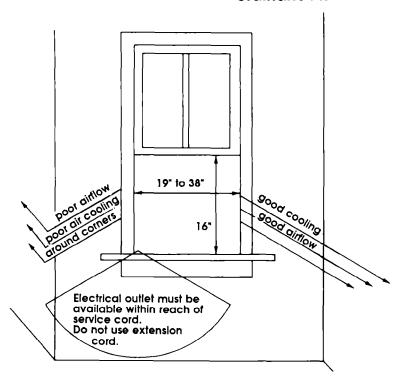
Check location where air conditioner will be installed. The location should provide:
