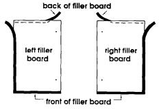
Apply seal strips to bottom and outside of of filler boards. The top seal goes on back side of filler board.
