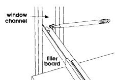
12. Lift sash and place side-mounting slides into top-mounting channel. Extend mounting slides outward into window channels. Pull air conditioner slightly forward until side mounting slides are tight against window channels. Mark and make 3/32' pilot holes for wood screws. Secure slides to window channels with wood screws.
