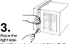
mounting angle over seal strip so that flange faces cabinet front. Insert sheet metal screws starting with bottom slot. Slide mounting angle downward until screws are in top of slots. Tighten screws. Repeat for left side-mounting angle, making sure flange faces cabinet front. (Note: Sidemounting angles may be factory-installed on some models.)
