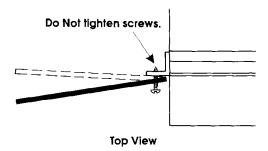
Pull cabinet part way out of window. Attach one filler board to side mounting angle using sheet metal screws. Do Not tighten screws at this time.
