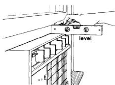
Lower window sash behind top-mounting channel. Place level on top of right side of cabinet. There should be a tilt to the outside of approximately one-half bubble. Place level on left side and check. If cabinet is not properly positioned, reposition or shim cabinet to provide proper tilt. Tighten filler board screws,
