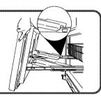
With drawer pulled out to full extension, insert lower basket by aligning tabs on both side of lower basket with notches in rail assembly.
