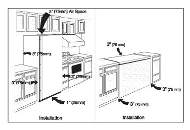
**NOTE:** The exterior walls of the freezer may become quite warm as the compressor works to transfer heat from the inside. Temperatures as much as 30° F warmer than room temperature can be expected. For this reason it is particularly important in hotter climates to allow enough space for air circulation around your freezer.
