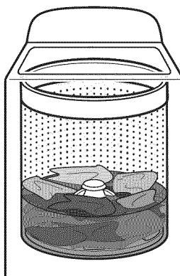
The most striking difference in your new washer is the low-water washplate wash system. The washer automatically adjusts the water level to the load size—no water level selector is needed.
