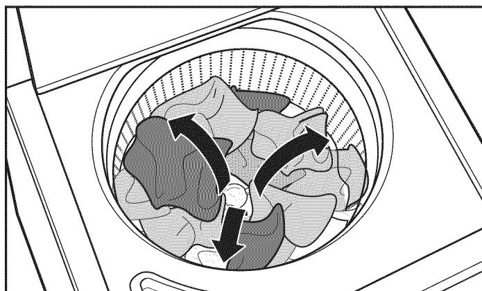
The washplate moves the load while water is added in small amounts until the load is wet. This low-water wash method uses less water and energy compared to a traditional agitator-style washer.
