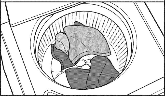
Load garments in loose heaps evenly around basket wall. Do not wrap large items such as sheets around the washplate; load them in loose piles around the sides of the basket. Try mixing different sized items to reduce tangling.
