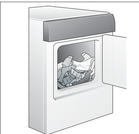
Fill dryer drum 1/3 to 1/2 full.
