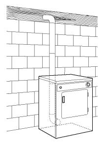
Rear exhaust installations for standard offset connections – (see pgs. 14-15).
