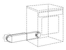
Vent system with one periscope (2" clearance)
