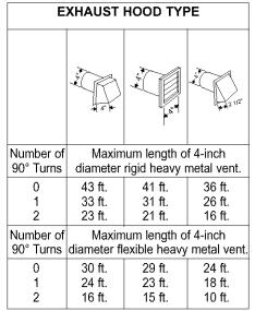
If a combination of rigid metal vent and flexible metal vent is used, use instructions for flexible metal vent (see p. 15).
