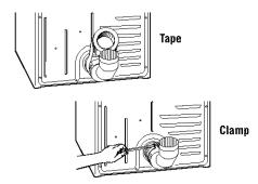
**STEP 4.** Connect vent to elbow. Tape the joint with duct tape. Tighten clamp.
