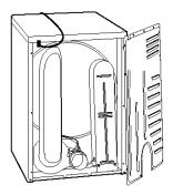
**STEP 3.** Remove lint from the dryer base with a soft brush or vacuum cleaner. Avoid damaging wires or electric thermostats.
