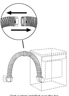
Vent system installed over the top with standard elbows
