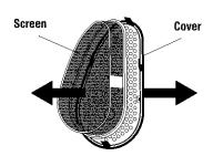
**STEP 3.** Roll lint off the screen with your fingers. Do not rinse or wash screen to remove lint. Wet lint is hard to remove.
