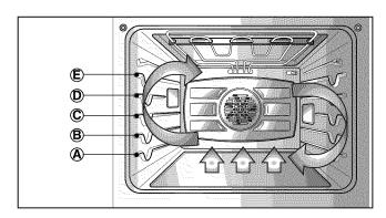
Convection baking uses a fan to circulate the oven's heat evenly and continuously within the oven. This improved heat distribution allows for even cooking and excellent results using multiple racks at the same time. Foods cooked on a single oven rack will generally cook faster and more evenly with Convection Bake. Multiple oven rack cooking may slightly increase cook times for some foods, but the overall result is time saved. Breads and pastries brown more evenly.
