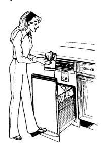
Lift and pull the handle or press the "Touch-Toe Bar" to open the drawer.
