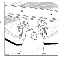
remove items in glass trap, grasp handle, lift out, empty and replace.
