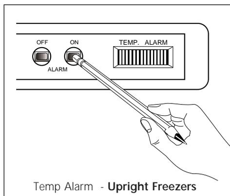
To activate the Temp Alarm, press the eraser end of a pencil, or a freezer key into the hole marked ON, moving the rocker switch. To deactivate the Temp Alarm, press the OFF switch.
