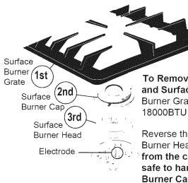
The Burner Grates, Burner Caps, Burner Heads, simmer plate and griddle should be routinely cleaned. Keeping the burner ports clean will prevent improper ignition and an uneven flame.
