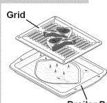
When broiling, heat radiates downward from the oven broiler for even coverage. The broil pan and broil pan insert used together allow dripping grease to drain and be kept away from the high heat of the oven broiler. **DO NOT** use the broil pan without the insert. **DO NOT cover the broil pan insert with foil.** The exposed grease could ignite.
