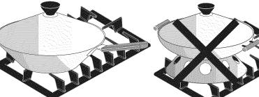
Proper use of flat-bottom wok on Surface Burner Grate Figure 2 Improper use of round-bottom wok on Surface Burner Grate Figure 3
