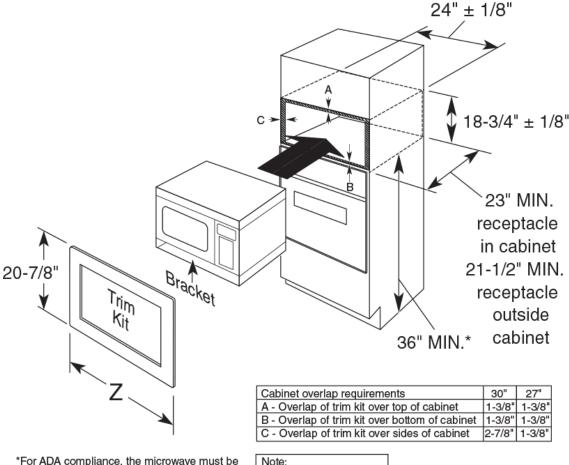
\*For ADA compliance, the microwave must be installed no higher than 37".
