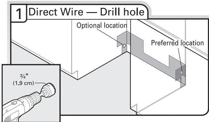
Drill a 3/4" (1.9 cm) hole in right-hand cabinet side or rear. See "Product and Cabinet Opening Dimensions" section.
