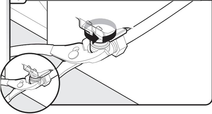
Be sure rubber washer is properly seated in fitting. Slide the 3/4" fitting up to the valve and hand tighten to avoid cross-threading. Hand tighten until the coupling is tight.
