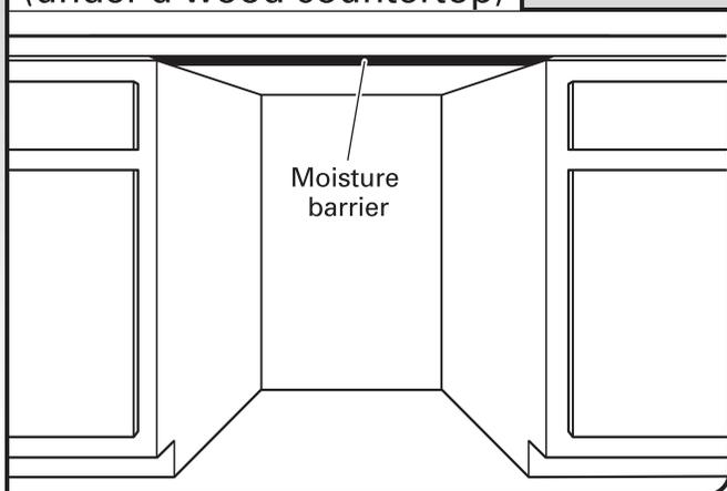
1. Make sure the area under the cabinet is clean and dry for installation of the moisture barrier.
