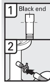
1. Connect black end of drain hose to waste tee and cut if needed.
