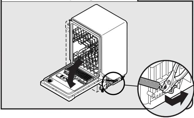
When door is unlatched and door opens by itself, move the tensioner to a lower numbered hole and replace the screw. Reattach door spring to rear leg.
