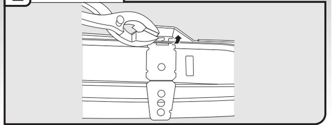
Using a pair of pliers, bend the tab down to secure the bracket in place. Repeat this step for the other side.
