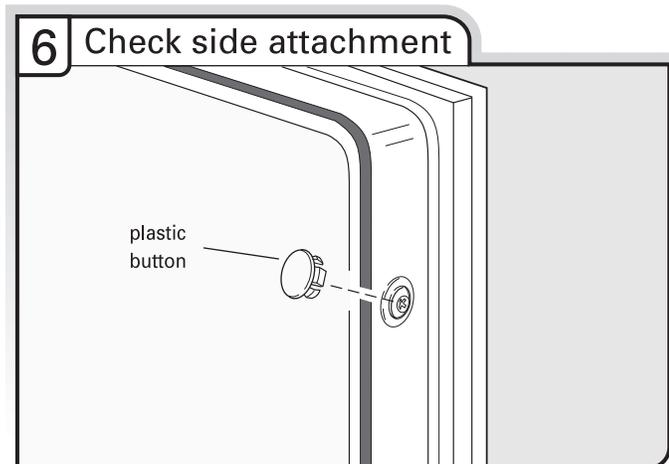
If securing with a side attachment, check that sides of door do not rub against the screw heads. If they do, dishwasher must be re-centered. When dishwasher is properly centered, replace plastic buttons.
