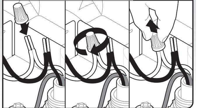
**NOTE:** Twist on wire connector. Gently tug on wires to be sure both are secured.
