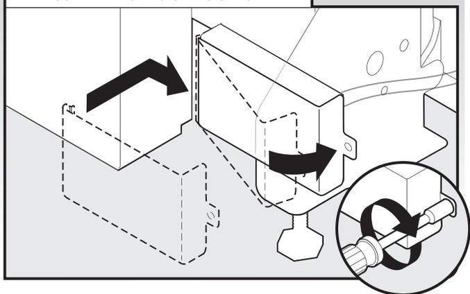
Place wires inside terminal box. Insert tabs on left side of cover. Make sure wires are tucked inside box. Close cover ensuring wires are not pinched. Use 1/4" nut driver and previously removed screw to secure cover.
