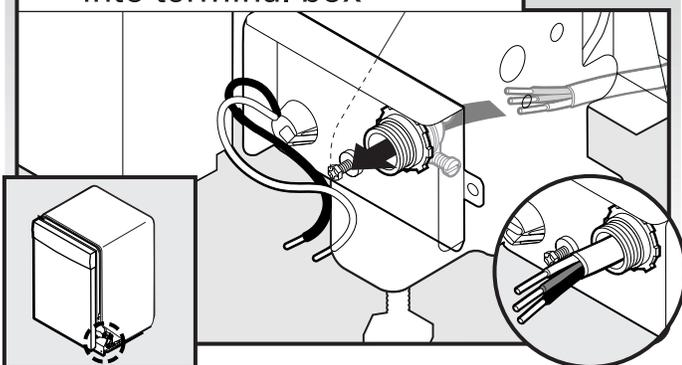
Route cable so that it does not touch dishwasher motor or lower part of dishwasher tub. Pull cable through UL Listed/CSA Approved strain relief in terminal box. Strain relief is not supplied with the dishwasher. Owner must purchase a 7/8" screw-in type strain relief.
