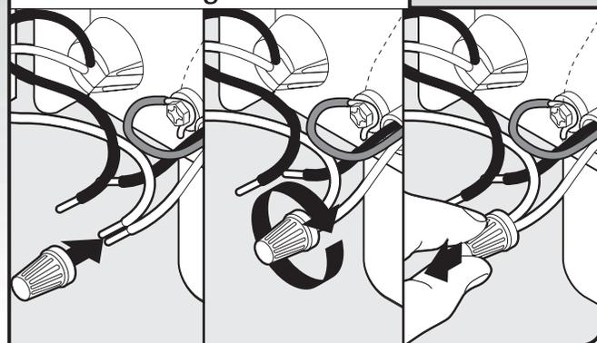
**NOTE:** Twist on UL Listed/CSA Approved wire connector. Gently tug on wires to be sure both are secured.
