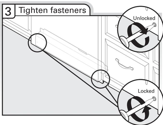
Using a flat-blade screwdriver, turn the fasteners ¼ turn to lock into place. The fasteners slot will be straight up and down when properly locked.
