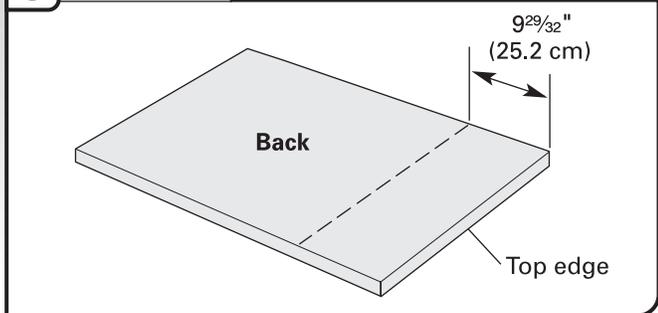
Measure  $9\frac{29}{32}$ " (25.2 cm) from top edge and mark a line on the back of customer-supplied custom panel. Position the outer panel on the back of the customer-supplied custom panel as shown, so that the top holes in the outer panel are on the line, and both panels are centered side to side.
