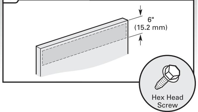
Attach outer panel to back of customer-supplied custom panel with the four #10-16 x  $\frac{3}{8}$ " hex head screws supplied in the literature package. Attach the handle. The handle should be centered on the front of the customer-supplied custom panel in the area shown.
