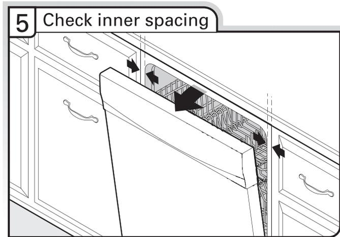
Open door and check that space between dishwasher cabinet opening and tub is equal on both sides. If spacing is not equal, loosen bracket screws secured and shift tub. Tighten bracket screws.
