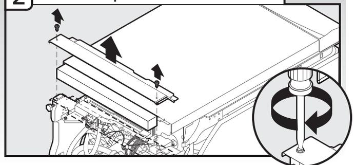
Using a flat-blade screwdriver, turn the plastic fasteners ¼ turn to unlock them. Remove panel. Do not remove tech sheet from access panel.
