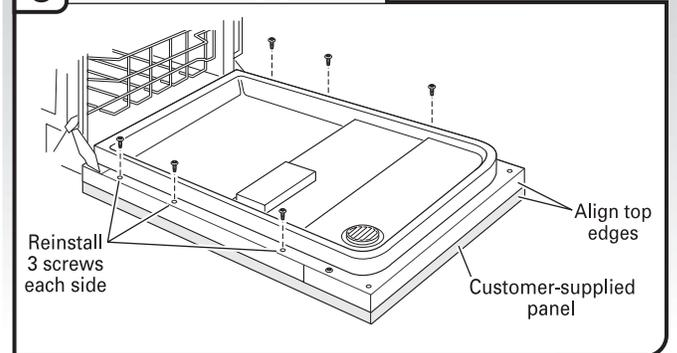
Attach the panel assembly to the door by reinstalling the three screws on each side; do not tighten completely. This reinstallation of the three screws will hold the panel assembly in place on the door frame.
