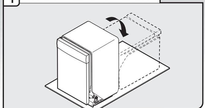
**Helpful Tip:** Place cardboard under dishwasher until installed in cabinet opening to avoid damaging floor covering. Do not use door panel as a worktable without first covering with a towel to avoid scratching the door panel.
