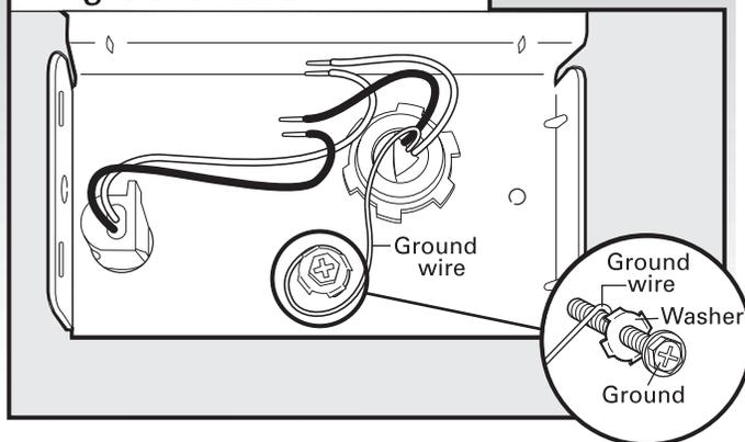
Form bare ground wire into a U-shaped hook. Wrap ground wire hook clockwise around ground connector screw and under the washer. Securely tighten ground connector.
