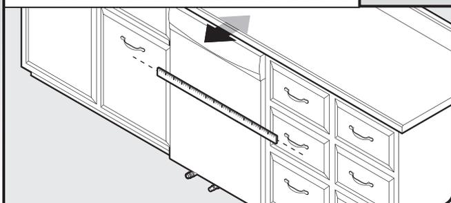
Align front of dishwasher door panel with front of cabinet doors. You may need to adjust alignment to be even with your cabinets.
