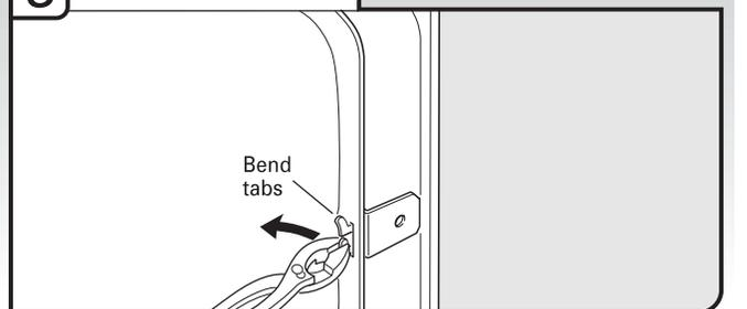
Push bracket into slot on the side of dishwasher, and bend tab in toward the side of the dishwasher so that it keeps the bracket in place. Repeat this step for the other side of the dishwasher.
