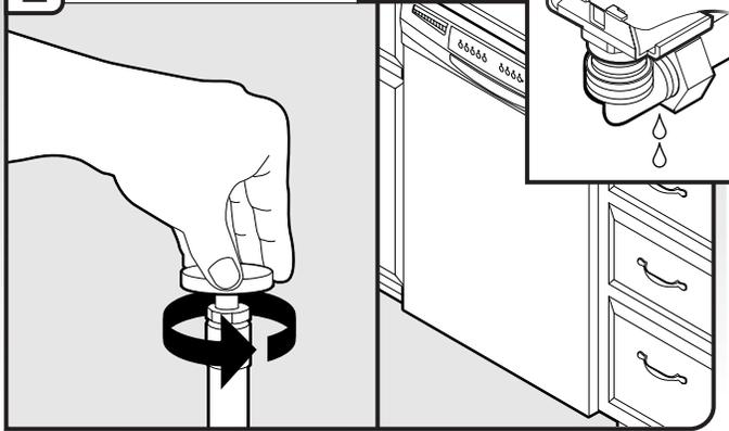
Place paper towel under 90° elbow fitting. Turn on water supply and check for leaks. If leak occurs, repeat previous step.
