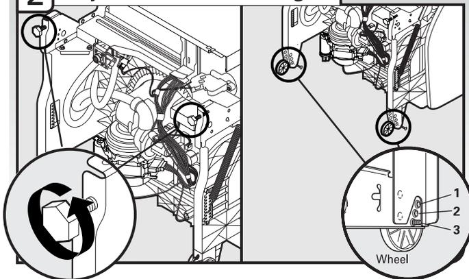
Turn both leveler legs to the same height. Put wheels in the required position determined from "Dishwasher Height Adjustment Chart."
