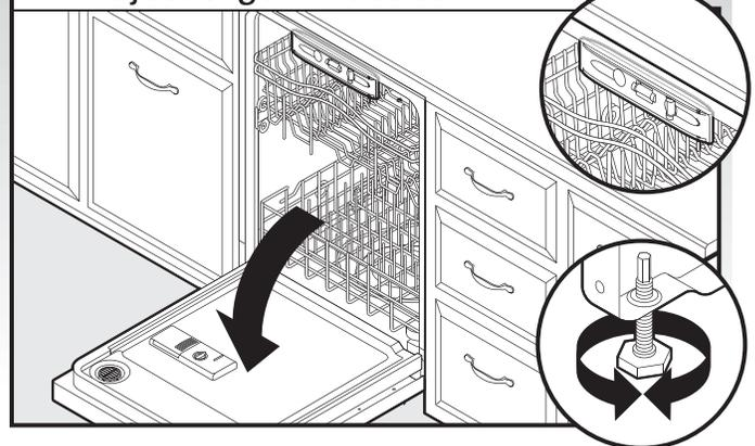
Place level against top front opening of tub. Check that dishwasher is level from side-to-side. If dishwasher is not level, adjust front legs up or down until dishwasher is level.
