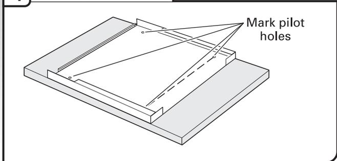
Mark all four hole locations; remove outer panel. Drill  $\frac{3}{32}$ " (2.4 mm) pilot holes  $\frac{1}{2}$ " (13 mm) deep in customer-supplied custom panel. Place the outer panel on the back of the customer-supplied custom panel; align holes.
