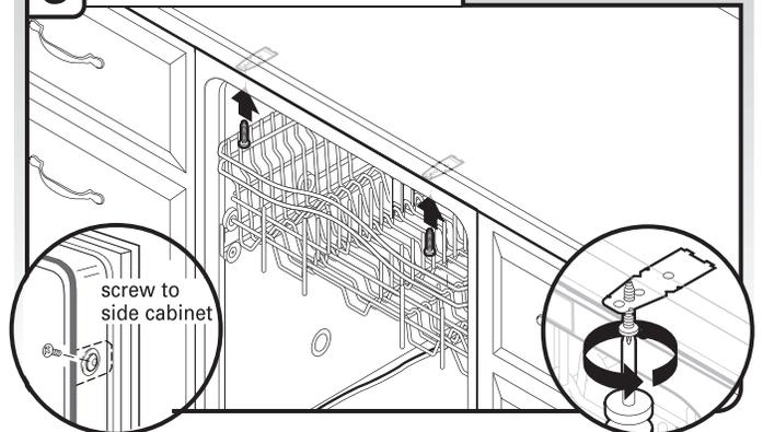
**NOTE:** Do not drop screws into bottom of dishwasher. If using side mounting, you must predrill (1/8" drill bit) pilot holes in cabinet to avoid splitting the wood before installing screws.
