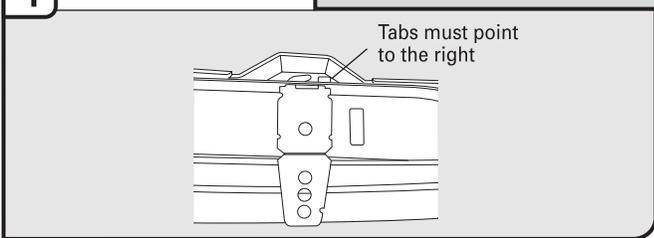
Remove the brackets from the package and insert into the open slots on the left and right-hand top of the dishwasher collar as shown.
