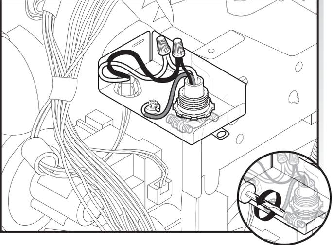
Tighten strain relief screws to secure cord.
