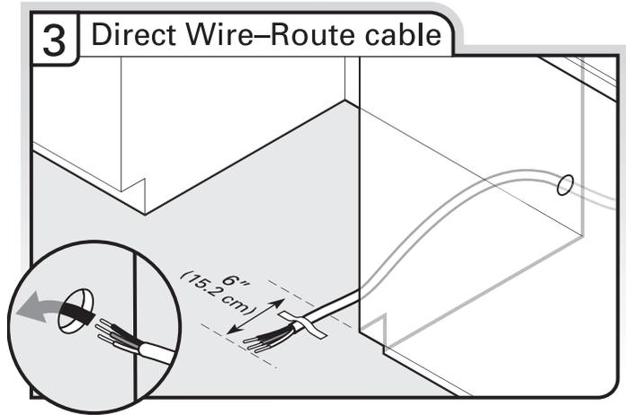
Route cable from power supply through cabinet hole (cable must extend to the right front side of cabinet opening). Tape cable to the floor in area shown. This will prohibit cable from moving when dishwasher is moved into cabinet opening.
