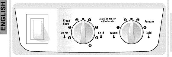
**IMPORTANT:** Turning the refrigerator temperature control to "0" turns off the compressor, but does not disconnect the power to the light bulb and other electrical components.
