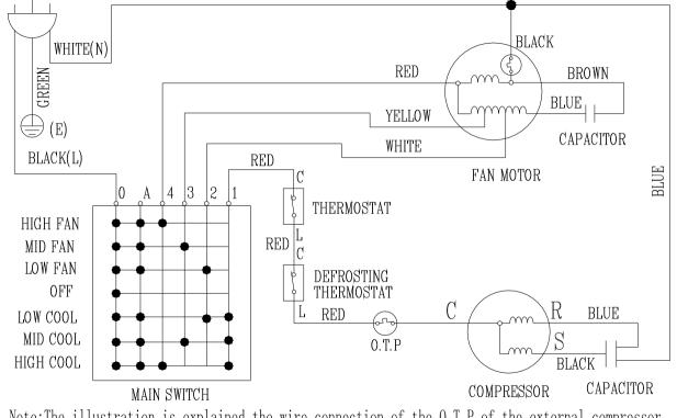
Note: The illustration is explained the wire connection of the O.T.P of the external compressor. For the internal compressor, the O.T.P has been connected with the compressor.
