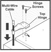
4 Remove the screws from the top hinge and pull the multi-wire cable through it. Lift the door off of the bottom hinge.
