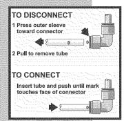
3 Detach the water tube from the connector located below the freezer door. The connector releases when you press its outer sleeve inward.
