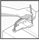
2 Trace lightly around the hinge with a pencil. This makes reinstallation easier.
