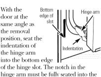
Fully open the door. If the door will not fully open, the indentation is not seated correctly in the bottom edge of the slot.
