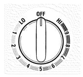
At both OFF and HI the control clicks into position. You may hear slight clicking sounds during cooking, indicating the control is maintaining your desired setting.
