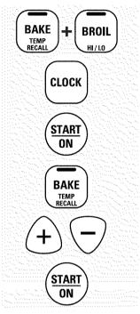
When the display shows ⊃ the oven is set in Sabbath. When the display shows ⊃ ⊂ the oven is baking/roasting.
