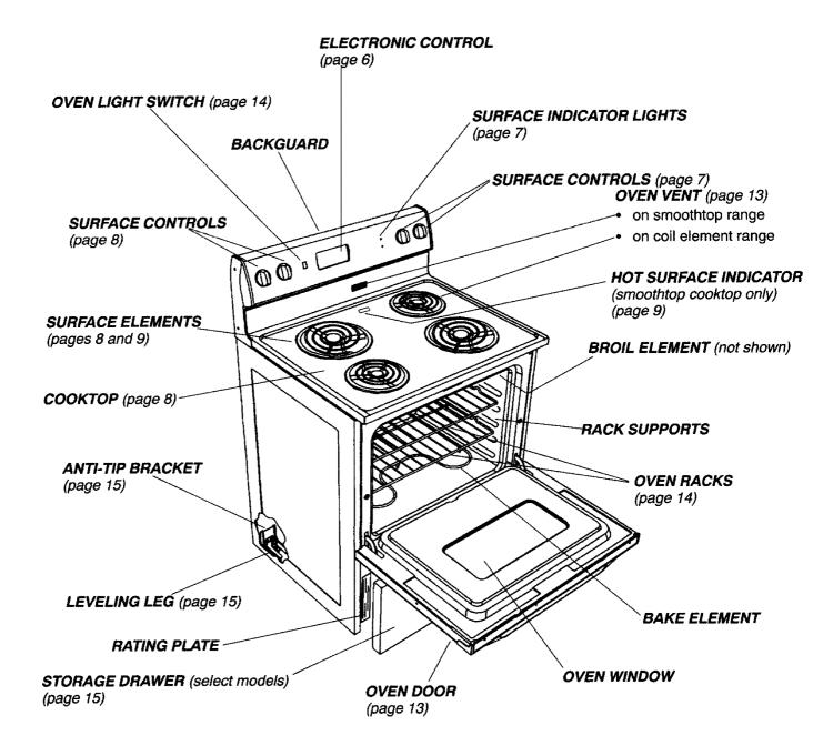
For slide-in and drop-in ranges: The surface control knobs and electronic control are on the manifold panel which is located above the oven door.
