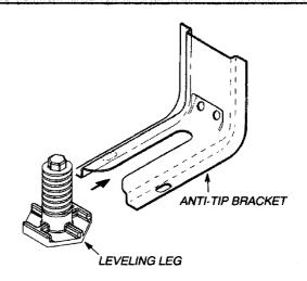
The installer should level the range when it is installed.
