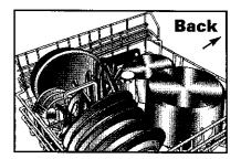
Convertible Tines (select models) in the back, right corner can be adjusted to provide narrow spacing for loading plates or wide spacing for loading deep bowls, pots or pans. Flip tines up for narrow spacing or down for wider spacing.
