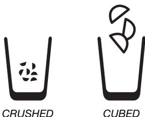
For crushed ice, cubes are crushed before being dispensed. This may cause a slight delay when dispensing crushed ice. Noise from the ice crusher is normal, and pieces of ice may vary in size. When changing from crushed to cubed, a few ounces of crushed ice will be dispensed along with the first cubes.
