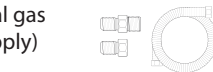
1/2" NPT union flare adapters (x2) and flexible gas supply line (gas dryer)
