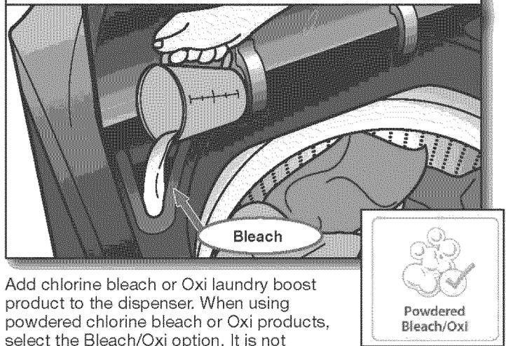
Add chlorine bleach or Oxi laundry boost product to the dispenser. When using powdered chlorine bleach or Oxi products, select the Bleach/Oxi option. It is not necessary to select the Oxi option when using liquid chlorine bleach or liquid Oxi products.
