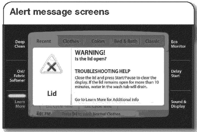
For many common problems that can be easily corrected without a service call, your washer will display an alert message with a code and explanation of the problem, as well as possible solutions.
