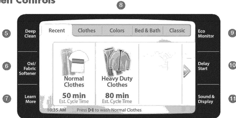
If a button along the side of the display has a green bar above it, that feature is currently activated. A blue bar indicates that you are in the display screen for that feature.
