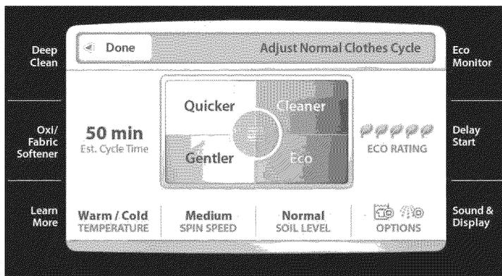
If you select Adjust Settings, you may manually choose and adjust each setting individually using the buttons across the bottom of the screen. If an option is not available, it will be grayed out and cannot be selected. You may also use the adjustment palette to calculate the best settings based on a quicker, gentler, cleaner, or more energy efficient wash cycle, or a combination of properties.
