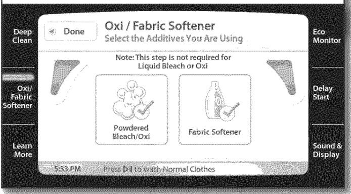
Touch the Oxi/Fabric Softener button to display the dispenser options page. Touch the Oxi-Boost and/or Fabric Softener icons to activate or deactivate each dispenser. When a dispenser is selected, a check mark will appear in the icon, and the dispenser name on the button will turn green. Once the desired dispensers are selected, touch Done to return to the main cycle screen.
