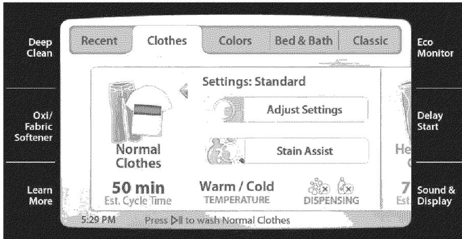
Once a cycle is selected, you will have the option of adjusting wash settings such as wash/rinse temperature, spin speed, and soil level. You may also add options such as Presoak and Extra Rinse, if available for that cycle. You can either go to the Adjust Settings menu to manually select settings for the load, or select Stain Assist, which will calculate the best settings for the stain.
