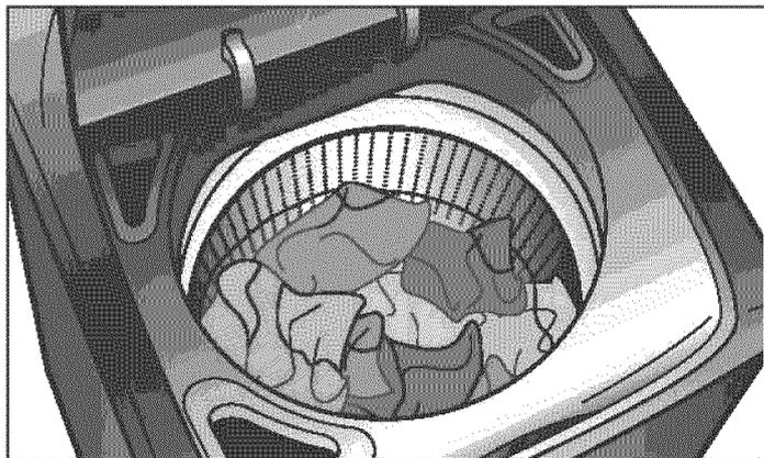
Water is added to the load while the basket turns slowly. As the washer dampens and moves the load, the level of clothes will settle in the basket. This is normal, and does not indicate that more clothes should be added.
