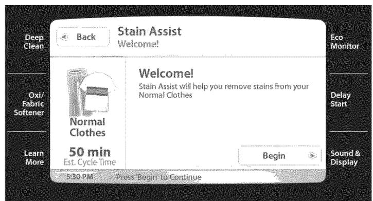
If you select Stain Assist, the washer will take you through 4 easy steps to determine the best settings for the stain. The washer will then calculate the best combination of temperature, wash time, and wash action for the stain and fabric.
