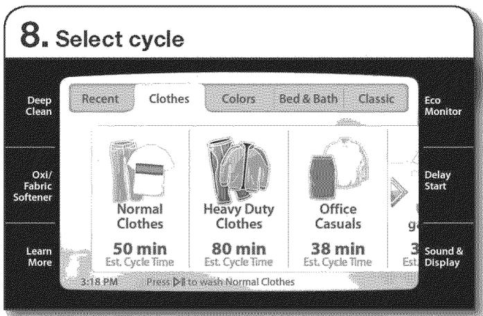
Use the touch screen to select the desired cycle. Cycles are grouped in tabs by type, and the last 7 cycles used will appear in the Recent tab. Touch the ◀ and ▶ arrows to scroll left or right.
