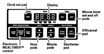
There are three parts in the oven control section:
