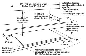
\*\* Note: 30" (76.2 cm) minimum when bottom of wood or metal cabinet is protected by not less than 1/4" flame retardant millboard covered with not less than No. 28 MSG sheet steel, 0.015" stainless steel, 0.024" aluminum or 0.020" copper.
