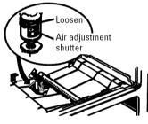
The shutter for the bottom (oven) burner is near the back wall behind the storage drawer. Remove the drawer. See the *Care and cleaning of the range* section.
