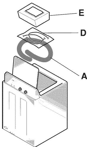
After the machine is in the home, remove remaining packing material/carton from washer.
