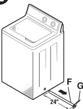
Move washer close to final position. Make sure there is at least a 24" clearance on right side of washer to remove shipping bar **F**. PULL SHIPPING BAR **F** OUT USING YELLOW PLASTIC HANDLE **G**. Keep bar so it can be reinstalled if washer is ever moved again.
