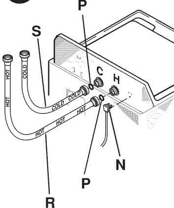
Remove electrical cord **N** from storage before installing water hoses. If not installed, install rubber washer **P** in one end of hot water hose **R**. Thread hot water hose **R** onto connection labeled **H** at top rear of washer. Hand tighten, plus an additional 1/8 turn with pliers.
