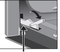
Lock engaged for door removal
