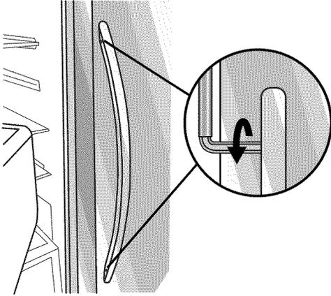
5. Using a clockwise motion, tighten the setscrew until it begins to contact the shoulder screw.
