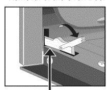
Lock engaged for door removal
