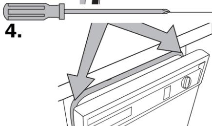
Open door about 3 inches (7.6 cm) and check that space between inner door and tub is equal on both sides. If spacing is not equal, loosen bracket screws and shift tub. Tighten bracket screws. Remove paper or towel from dishwasher.
