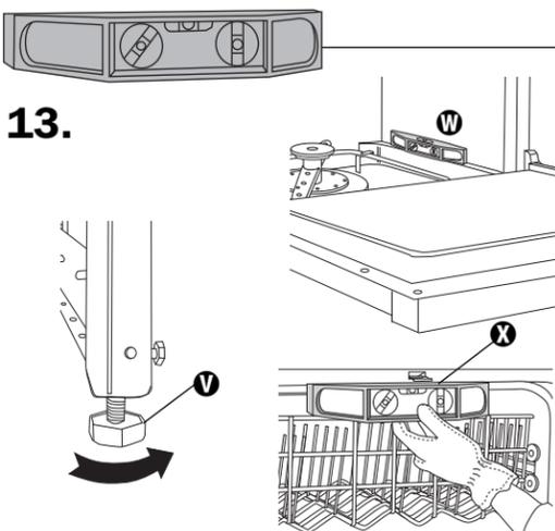
13. Check that leveling legs **V** are firmly against the floor. Place level on the rack guide **W** on one side of the dishwasher tub. Check that dishwasher is level from front to back. Adjust leveling leg or add shims under rear wheel until dishwasher is level. Repeat for other side of dishwasher. Place level against top front opening of tub **X**. Check that dishwasher is level from side to side. If dishwasher is not level, adjust front legs up or down until dishwasher is level.
