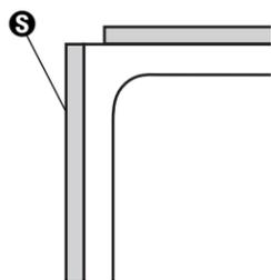
**NOTE:** If dishwasher has been moved and the new cabinet opening is 24 inches (61 cm) or more, pull dishwasher partially out of cabinet. Align top edge of tub collar **S** with top of dishwasher tub side flange **S**. Snap tub collar onto side flange **S**. Check that tub collar is securely attached to dishwasher. Repeat on other side.
