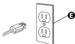
Install a mating, three-prong, grounding-type wall receptacle **E** in the cabinet next to the dishwasher opening. Go to step 6.
