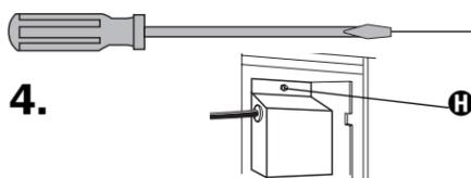
Reinstall terminal box cover **H** with wires inside terminal box. Go to step 5.
