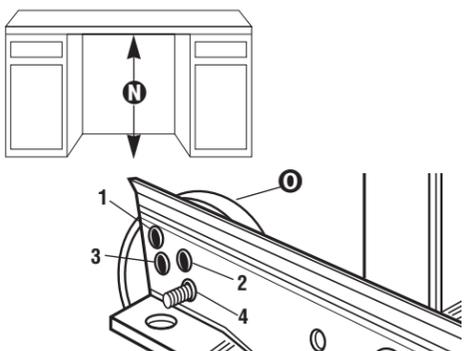
Measure height of cabinet opening from underside of countertop to floor where dishwasher will be installed **N** (you need the lowest point). Check chart for that height opening. Put wheels **O** in the required position.
