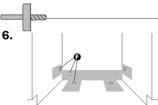
Cut a 1/2" (1.3 cm) minimum hole **F** in left-hand cabinet side, rear or floor. Optional locations are shown.
