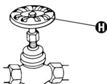
Turn shutoff valve **H** to "ON" position. Flush water into a bucket to get rid of particles that may clog the inlet valve.
