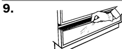
Carefully slide color access panel and spacer upwards and remove. Save color access panel and spacer for future use.
