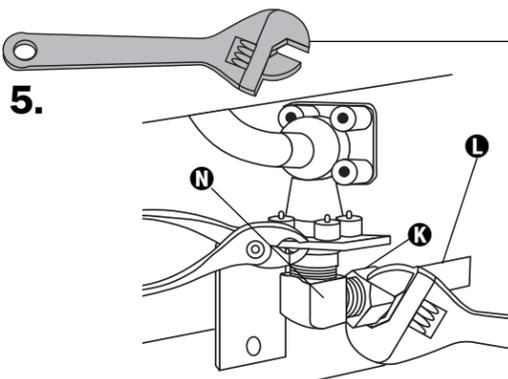
To prevent vibration during operation, route the water supply line so that it does not touch the dishwasher base, frame or motor.
