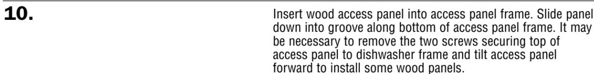
Insert wood access panel into access panel frame. Slide panel down into groove along bottom of access panel frame. It may be necessary to remove the two screws securing top of access panel to dishwasher frame and tilt access panel forward to install some wood panels.
