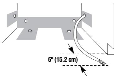
Run other end of wire through cabinet hole. Cable must extend to the right front of cabinet opening. Go to step 6.
