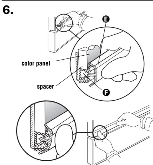
6. Snap one end of retainer into channel **E** as shown. Push inward while sliding thumb along full length of retainer **F**.
