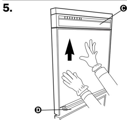
5. Push in on door panel(s) near the top and slide panel(s) and spacer up inside bottom of control console **C**, allowing panel(s) to rest on channel at bottom of door **D**.
