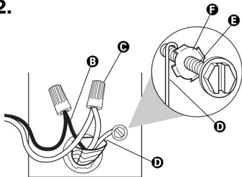
Connect the wires **B** as follows using twist-on connectors **C** sized to connect direct wire to 16-gauge dishwasher wire:
