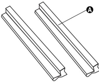
Put dishwasher corner posts **A** behind dishwasher. Grasp sides of dishwasher door frame and put dishwasher on its back.
