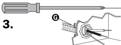
Tighten clamp connector or conduit connector screws **G**.
