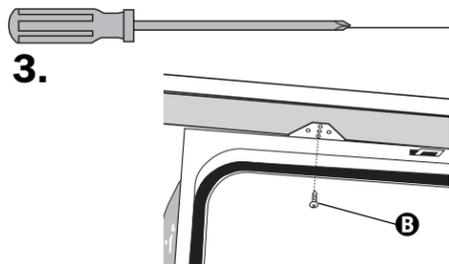
Secure dishwasher to countertop with two, No. 10 x 1/2" Phillips-head screws **B**. The dishwasher **MUST** be secured to keep it from tipping when door is opened. Do Not drop screws into bottom of dishwasher.
