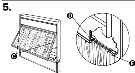
Insert top of wood door panel between sides of door frame about 3" (7.5 cm) below console **C**. Rotate wood door panel down against dishwasher door. Slide top edge of wood door panel under bottom edge of console **D**. Press lower portion of wood door panel in place between sides of door frame **E**, allowing wood door panel to rest on channel at bottom.
