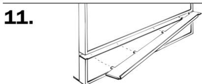
Line up edges of top trim with sides of access panel frame. Tilt back of trim down and slide into place. Snap front of trim down to cover top edge of wood access panel.
