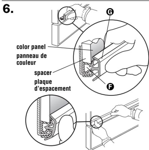
Snap one end of retainer into channel **F** as shown. Push inward while sliding thumb along full length of retainer **G**.
