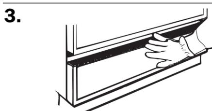
3. With desired color facing out, bow access panel and insert it into access panel frame. Slide panel down into groove along bottom of access panel frame.
