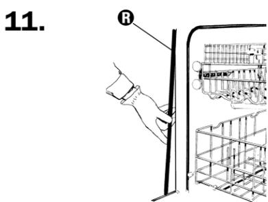
11. If dishwasher is equipped with a tub collar **S** and does not fit in cabinet opening or cabinet opening is less than 24 inches (61 cm) wide, partially pull dishwasher out of cabinet. Carefully pull the two side tub collars off of dishwasher and save. Push dishwasher back into cabinet opening.
