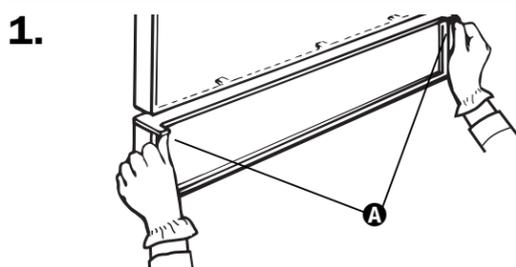
1. Wear gloves and handle panels carefully. Push up with thumbs on each end of access panel top trim **A** to unsnap trim. Remove top trim and set it aside.
