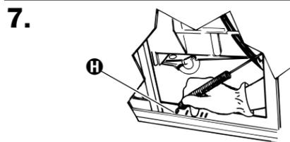
Check door for proper operation. Door should close easily without slamming and open with its own weight. If necessary, close door and adjust both door springs by moving spring ends **H** to different holes in base.
