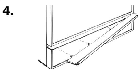
4. Line up edges of top trim with sides of access panel frame. Tilt back of trim down and slide into place. Snap front of trim down to cover top edge of access panel.
