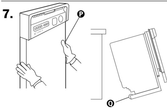
7. Grasp the dishwasher door frame **P**. Tilt dishwasher backwards on wheels **Q**. Move dishwasher close to cabinet opening. Do not push on dishwasher panels or console—they may dent.
