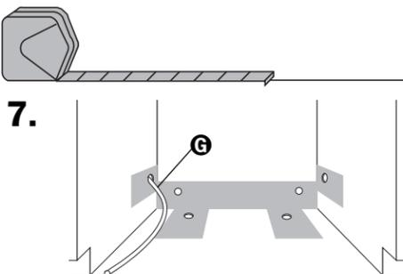
Measure overall length of copper tubing **G** required. Attach copper tubing to water line with manual shutoff valve. Carefully feed copper tubing through hole in cabinet (copper tubing will bend and kink easily) until it is far enough into the cabinet opening to connect it to dishwasher inlet on the front left of dishwasher.
