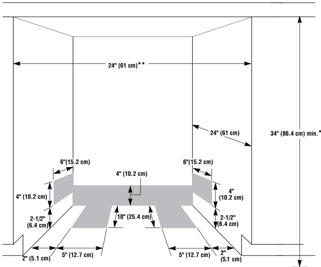
Cut openings in shaded area of cabinet walls or floor as specified in chart:
