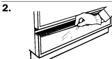
2. Carefully slide color access panel upwards and remove. **Do Not remove spacer.**
