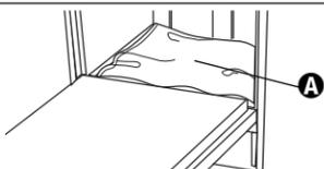
Open dishwasher door and place towel **A** over pump assembly and spray arm of dishwasher. This will prevent screws from falling into pump area when securing dishwasher to countertop.
