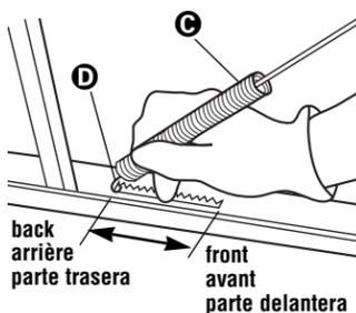
Open and close the door several times. The door should open and close easily. If the door closes too quickly, decrease the spring **C** tension by moving the spring end **D** toward the front of the dishwasher. If the door falls open, increase the spring tension by moving the spring end toward the back of the dishwasher. Springs should be in the same notches on left and right sides.
