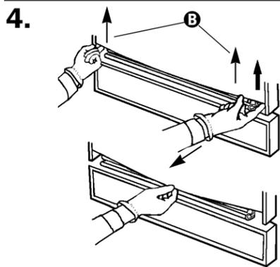
Lift door panel(s) at outer edges **B**. Use one hand to bow bottom of panel(s). Remove panel(s) and spacer. Save panel(s) and spacer for future use.
