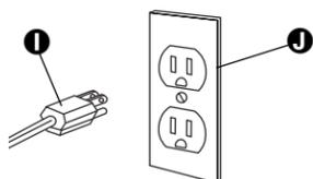
Plug power supply cord ❶ into mating grounded outlet ❷. Go to step 5.
