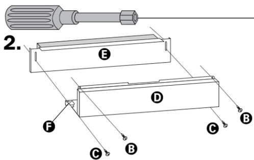
Remove two top screws **B** and two bottom screws **C** attaching access panel **D** and lower panel **E** to dishwasher using a 1/4" hex socket, nut driver or Phillips screwdriver. Remove panels and set panels aside on a protective surface. Check that grounding clip **F** stays attached to access panel.
